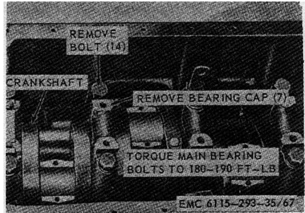
Figure 67. Crankshaft and main bearings, removal and installation.
